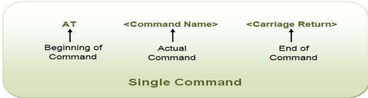
Fig 3.1: Using a Single AT Command
